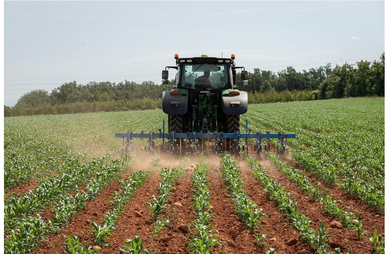
Mechanical weeding in maize @ INRAE
